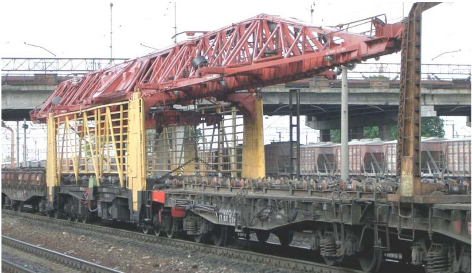
track-laying crane UK-25, converted for electric operation
