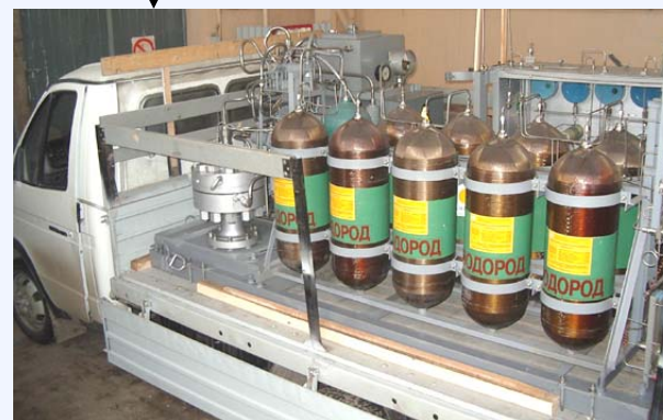
Hydrogen delivery in cylinders
