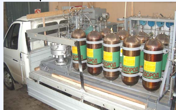
Hydrogen delivery in cylinders
