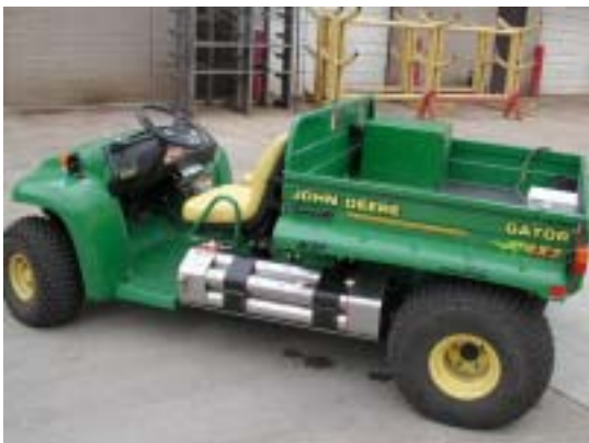
Fuel Cell Vehicle with MH Storage
